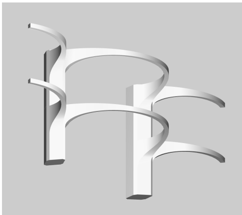
Figure 3: ring beam and haunch detail at perimeter columns, Marina City towers [drawing done later by author]
